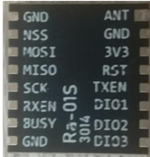
Figure 4 Ra-01S Pin Diagram
