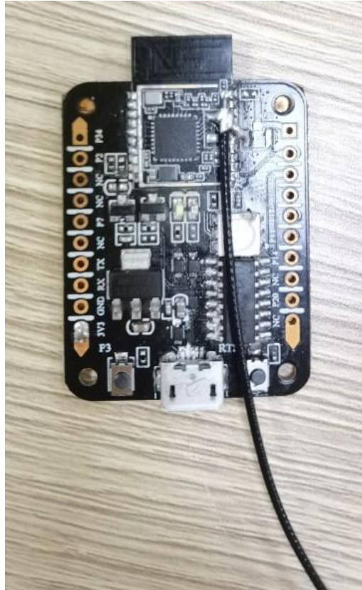
Figure 7 schematic diagram of antenna test prototype
