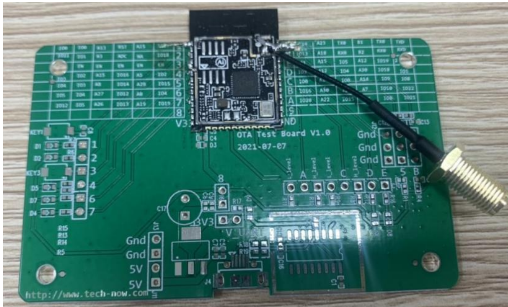
Figure 8 schematic diagram of antenna test prototype
