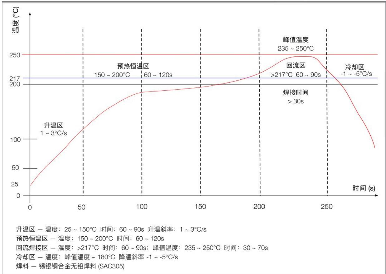
Figure 12 Reflow weld curve diagram
