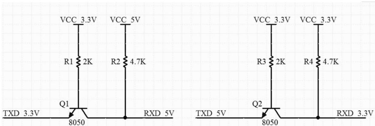
Figure11 Electrical Level conversion circuit
