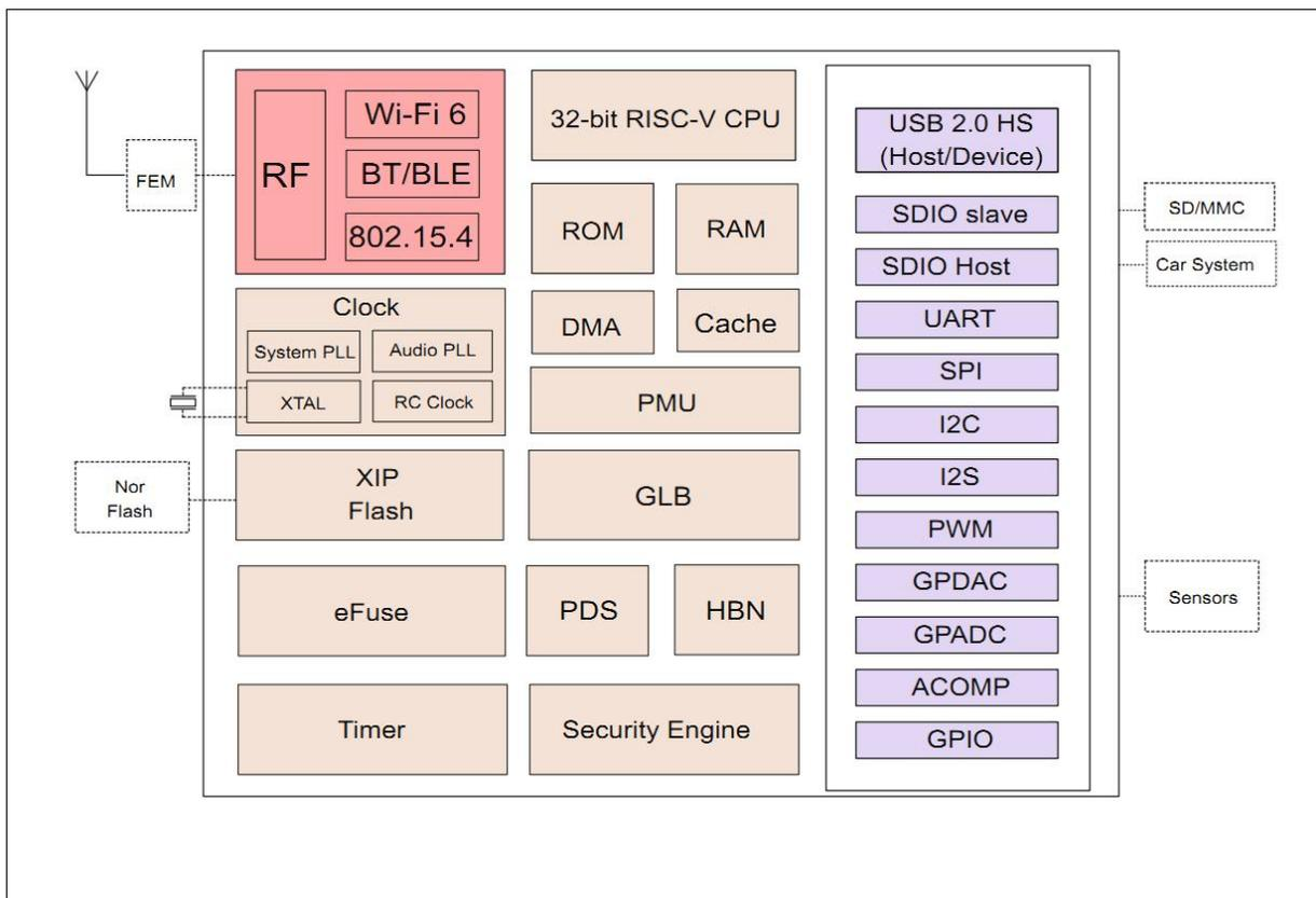
**Figure 1 Main chip block diagram**
