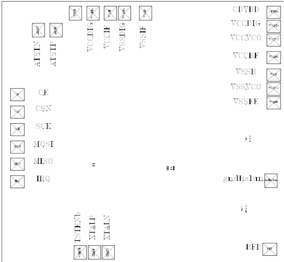
**Figure 12 Bonding diagram**
