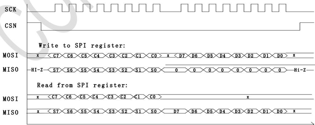
**Figure 6 SPI timing**
