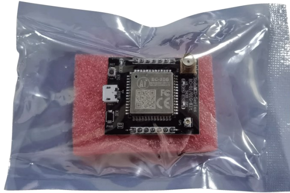
Figure 11 Packing diagram of an ESD bag
