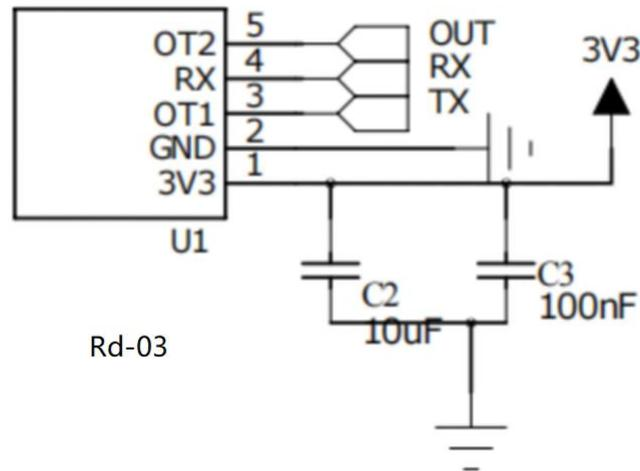
Figure 7 Application guide circuit
