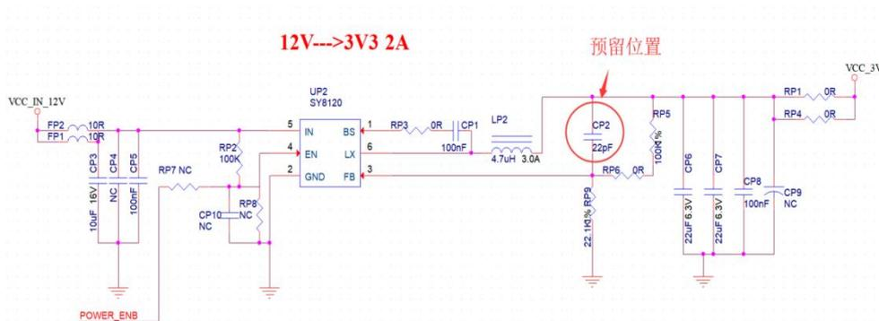
Figure 15 DC-DC step-down circuit diagram
