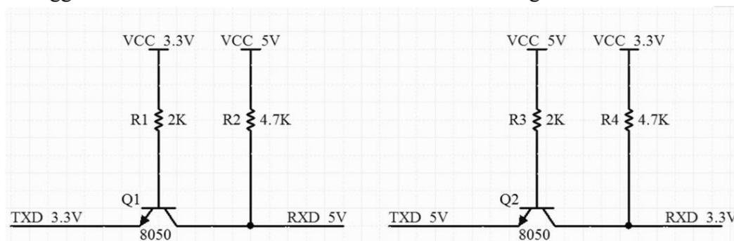
Figure 16 Level switching circuit
