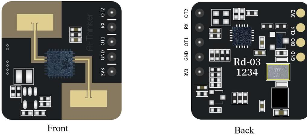
Figure 5 Pin diagram
