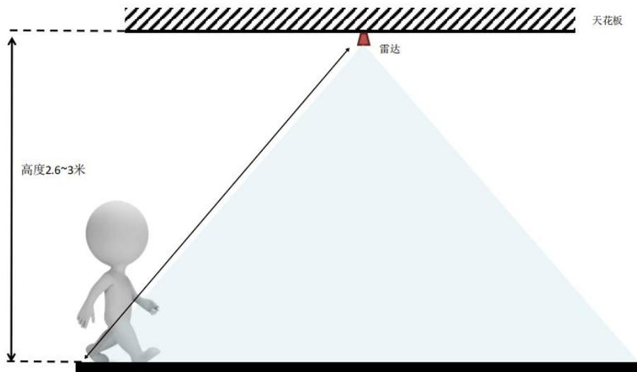
Figure 9 Schematic diagram of mounting the roof
