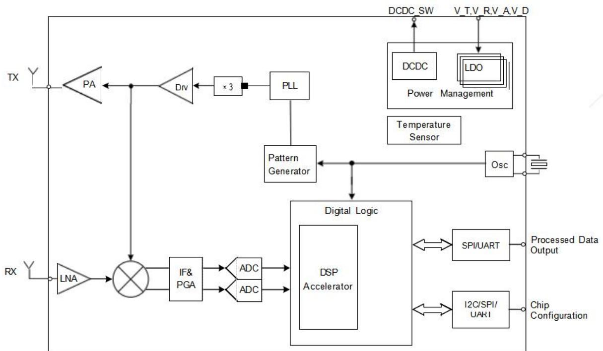
Figure 1 S3KM1110 architecture diagram
