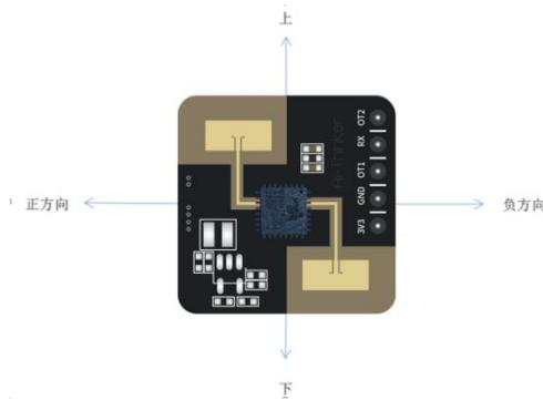
Figure 13 Schematic diagram of wall-mounting direction
