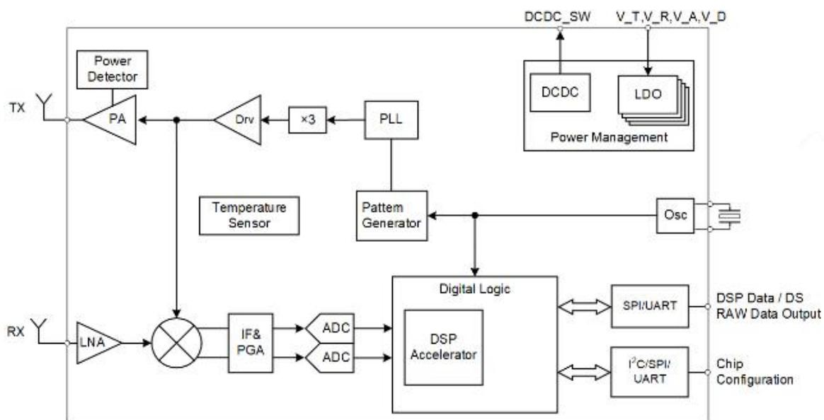
Figure 1 ICL1112 chip architecture
