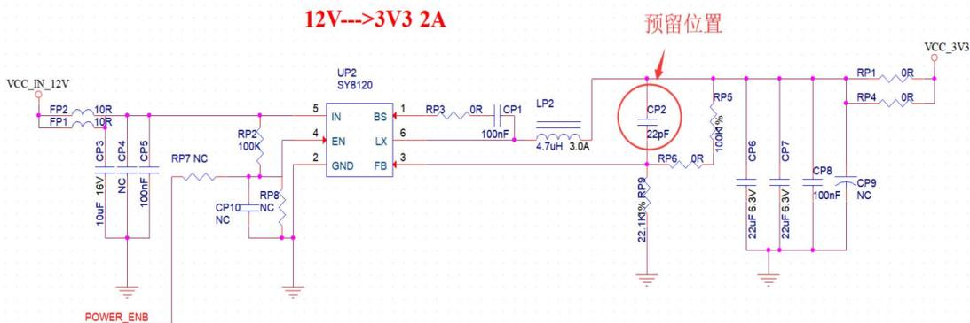
Figure 13 DC-DC step-down circuit diagram
