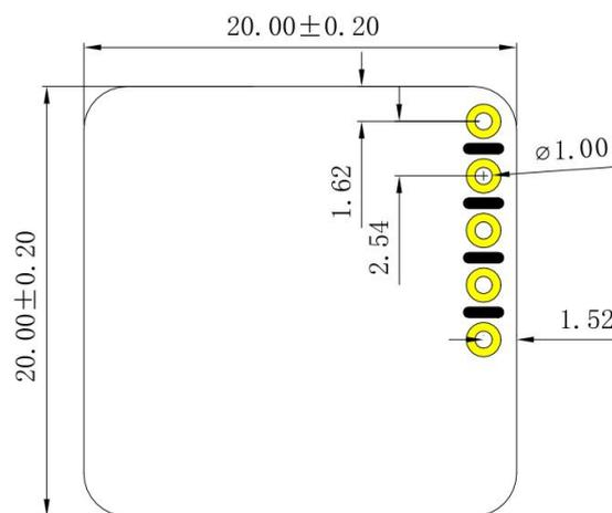
Figure 9 recommend PCB package size
