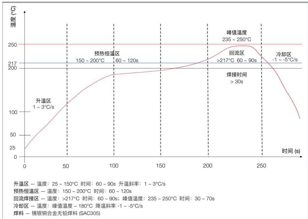
Figure 15 Reflow welding curve
