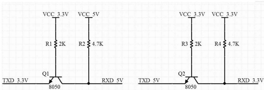
**Figure 14 level conversion circuit**
