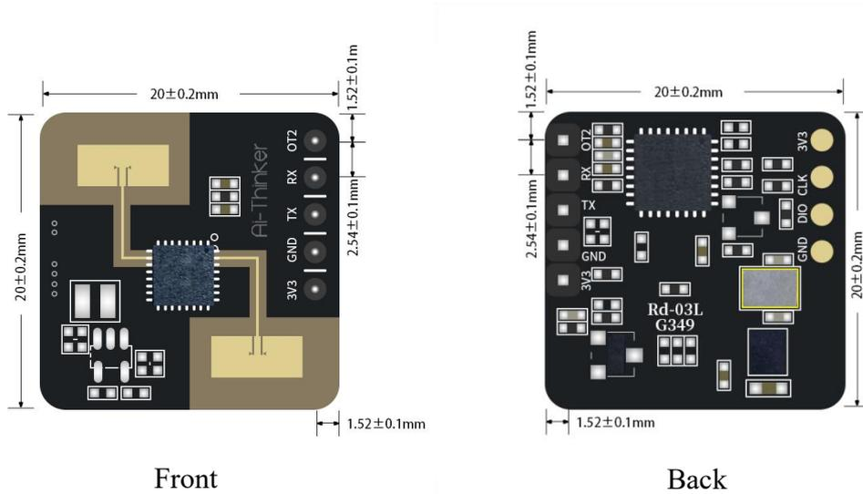
Figure 5 Dimension Diagram
