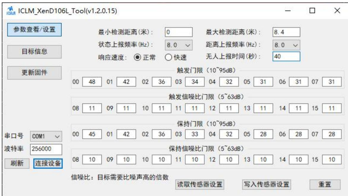
Figure 3 radar setting parameter diagram
