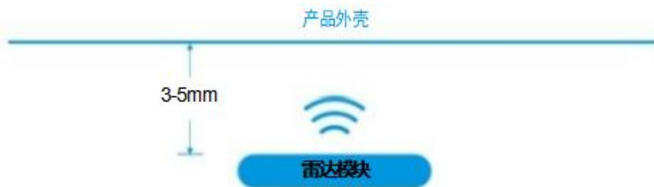
Figure10 Distance between the antenna surface and the product shell
