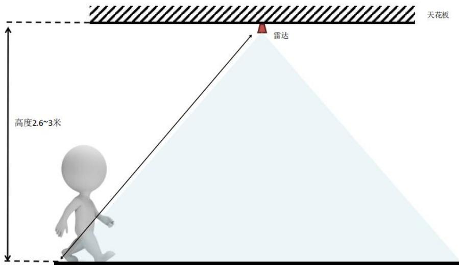
Figure 10 Schematic diagram of the top-hanging installation
