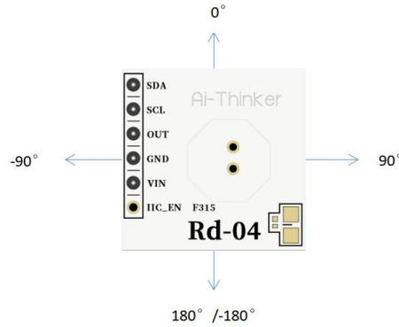
Figure 11 Direction diagram of the module for top-hanging
