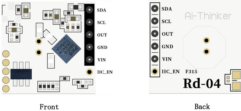
**Figure5 Pin schematic diagram**
