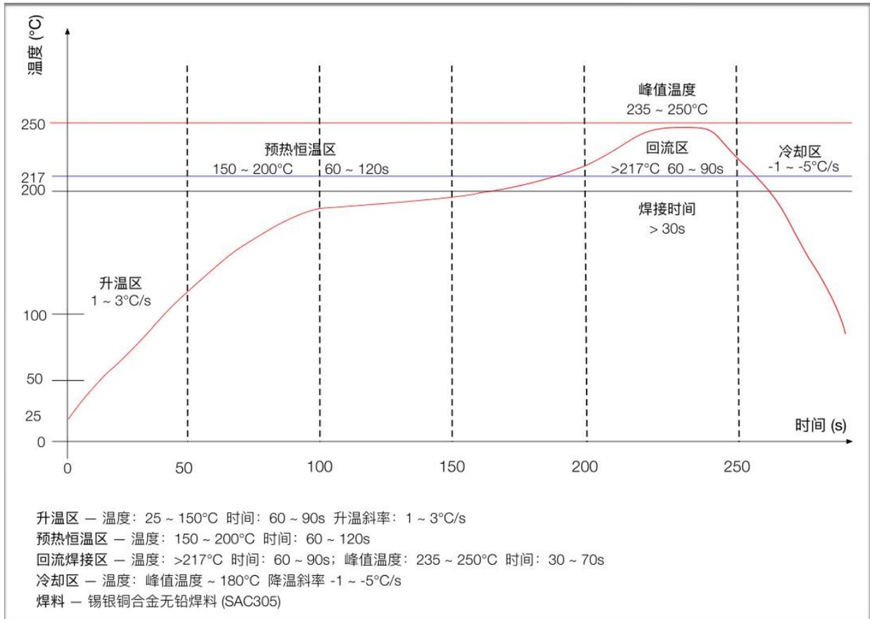
Figure18 Reflow Soldering Curve
