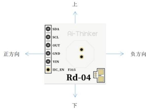
Figure 14 Direction diagram of the module for wall-hanging
