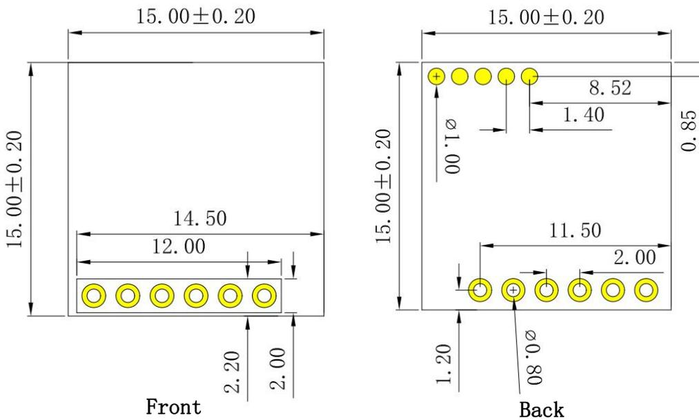
Figure 4 Dimension diagram
