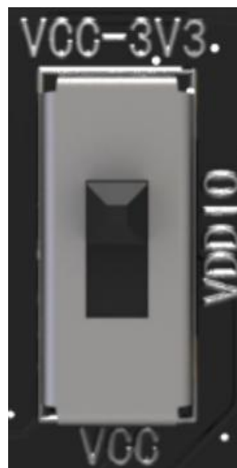
Figure 9 Schematic diagram of the power selection switch
